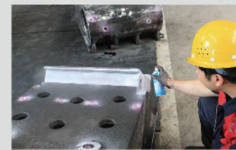
渗透探伤 Penetrant testing
